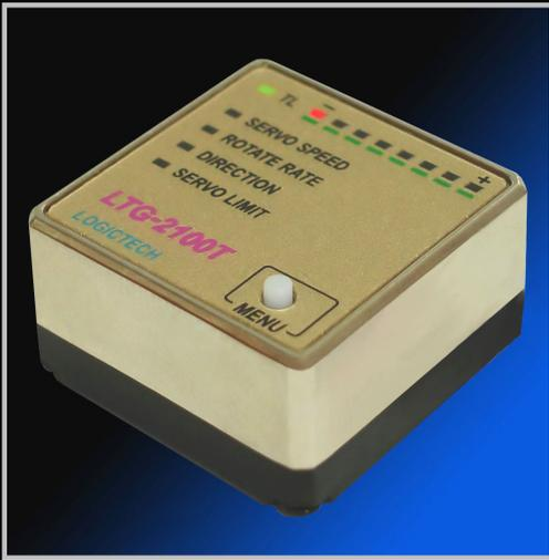
LTG-2100T is High Performance Gyro for EP Helicopter.
