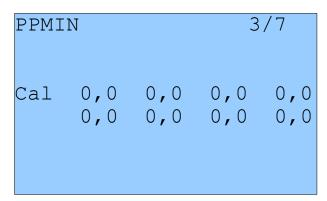
This menu allows you to calibrate the mid point for the input PPM channels.
