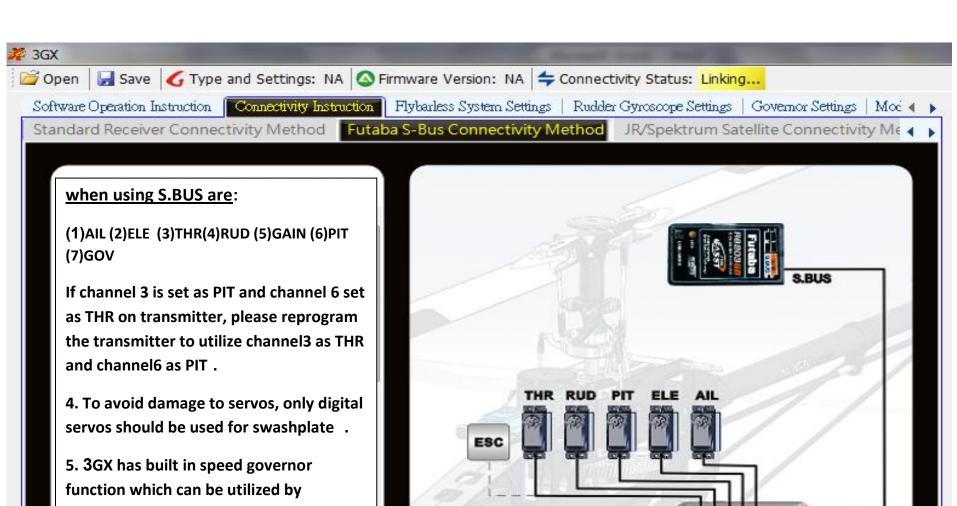
5. 3GX has built in speed governor function which can be utilized by purchasing the optional speed sensor.
