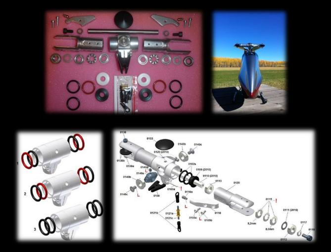
Two kind of Damping case can be used (black from the kit or white from the old 2009 kit) +Dumping O Rings that can stiff the head of the HELI in six different levels. I assembled the TDR with the old white Dumping case with a combination of option No.2 (orange dumpers to central hub and black ones outside).
