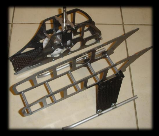
Connecting the frames to each other and adding the Gyro sensor carbon plate at the back of the HELI.
