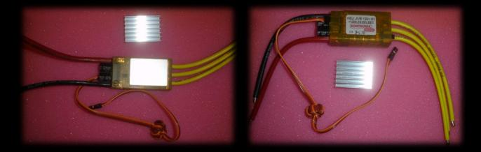
According to KONTRONIK gluing a Heat sink to the controller can double the current consumption that this controller can deliver. It's important on such a HELI that its canopy completely covers the Engine and the controller during Flight.
