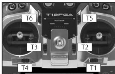
This transmitter is equipped with six digital trims. Each time you press a trim button, the trim position moves one step. If you continue pressing it, the trim position starts to move faster. In addition, when the trim position returns to the center, the tone will change. You can always monitor trim positions by graphics on the screen.
