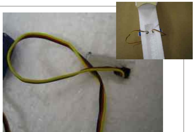
Step 20: Feed the servo plug through to the radio compartment. Seat the servo in the hole and glue the lugs with CA glue.
