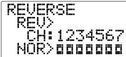
Except with CCPM helicopters, always complete your servo reversing *prior* to any other programming. If you use pre-built ACRO functions that control multiple servos, such as FLAPERON or V-TAIL, it may be confusing to tell whether the *servo* needs to be reversed or a setting in the *function* needs to be reversed. See the instructions for each specialized function for further details.
