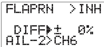
The FLAPERON mixing function uses one servo on each of the two ailerons, *and* uses them for both aileron and flap function. For flap effect, the ailerons raise/lower simultaneously. Of course, aileron function (moving in opposite directions) is also performed.
