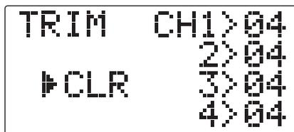
The 7CA has digital trims which are different from conventional mechanical trim sliders. Each **TRIM LEVER** is actually a two-direction switch. Each time the **TRIM LEVER** is pressed, the trim is changed a selected amount. When you hold the **TRIM LEVER**, the trim speed increases. The current trim position is graphically displayed on the start up screen. The TRIM submenu includes two functions that are used to manage the trim options.
