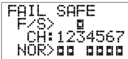
**FailSafe (F/S):** instructs a PCM receiver what to do in the event radio interference is received.
