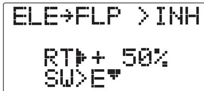
ELEV-FLAP mixing is the first pre-programmed mix we'll cover. This mix makes the flaps drop or rise whenever the **ELEVATOR STICK** is moved. It is most commonly used to make tighter pylon turns or squarer corners in maneuvers. In most cases, the flaps droop (are lowered) when up elevator is commanded.
