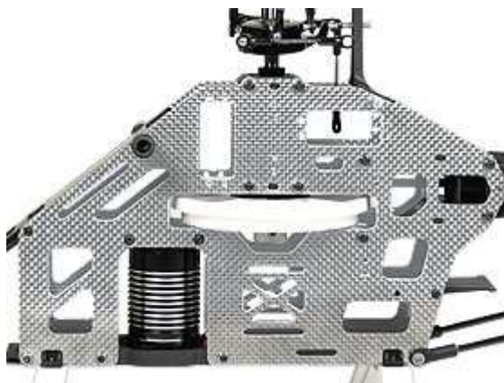
Focus Shot3(New-sturdy lightweight main frame/1.6mm) Focus Shot4(Fiberglass painted canopy)
