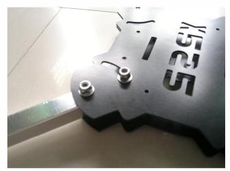
9. Install the four square aluminum tubes successively, finish assembly by fixing the M4 nut and M4\*25 screws. The square aluminum tubes can be moved by adjusting the screws.
