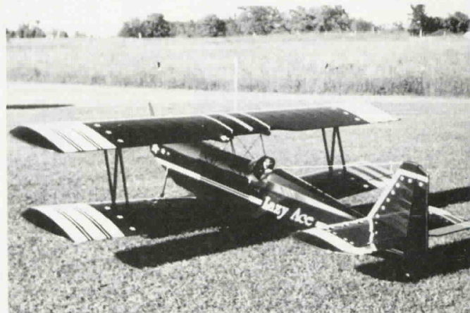
Lazy Ace built by Dennis Fahselt. O.S. 90 2-stroke engine. Going to add smoke system.
