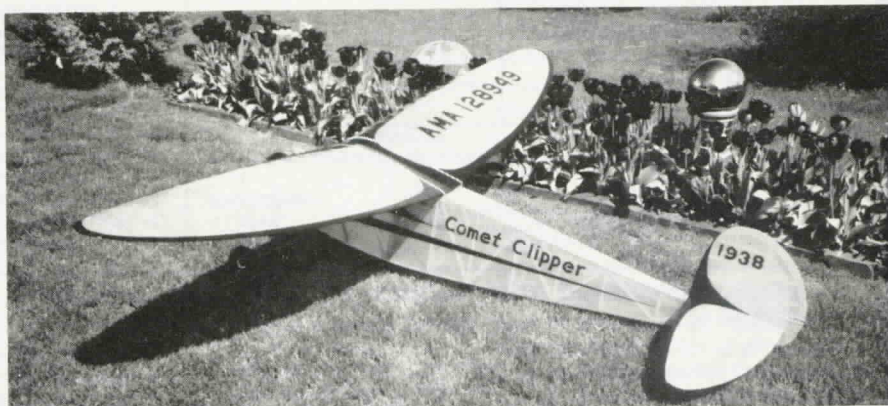
Ten foot span Comet Clipper, scaled up from John Pond plans. Built by A.J. Serfass in Brookfield, Missouri. Plans to add 60" floats to it. ST .75 engine, 10 lbs. all-up weight, should be magnificent in the air.
