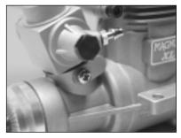
of the carburetor into the crankcase, being careful to keep the carburetor perpendicular to the front of the engine. Using your thumb, push down firmly on the carburetor so the base of the carburetor sets completely into the crankcase. An o-ring is installed on the carburetor throat to seal the joint. While holding the carburetor
