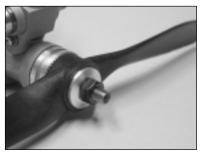
Running an engine using an outof-balance propeller can lead to excessive vibration which will result in excessive stress and wear on both the engine and the airframe. Balance the propeller using the method recommended by the propeller manufacturer. Several products are available to properly balance propellers. Ask
