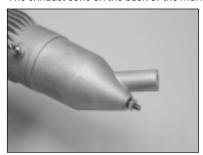
the installation of your particular application. To adjust the exhaust cone, loosen the retaining nut using an adjustable wrench. Rotate the cone to the desired angle and tighten the retaining nut completely while holding the axial bolt in place from the front of the muffler, using a flat blade screwdriver. It is important to
