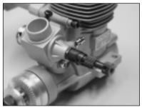
your engine. You can easily mount the needle valve in the side of the carburetor if you wish.
