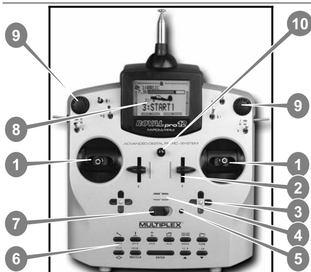
Fig. 9.1.1.: Front face of transmitter (Switches K and P retro-fitted; not included as standard.)
