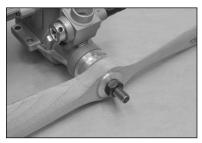
Using a 1/4" drill bit or a propeller reamer, enlarge the hole in the propeller hub to fit the crankshaft. Slide the propeller onto the crankshaft, up against the drive washer, then slide the propeller washer up against the propeller and thread the propeller nut into place. Tighten the propeller nut
