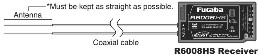
Futaba's dual antenna diversity then seamlessly selects the best signal reception between these antennas to ensure that there is no loss of signal.
