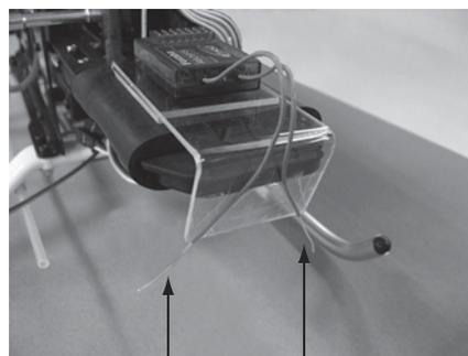
\*The two antennas should be placed at 90 degrees to each other.
