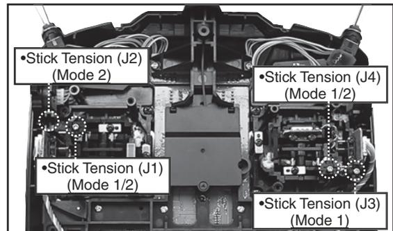
2. Use a small Phillips screwdriver to adjust the spring strength as you prefer by turning the adjusting screw of the stick you want to adjust.
